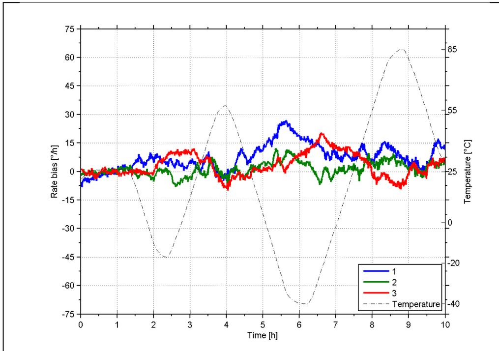
Figure 6-5: Typical Bias drift over temperature
