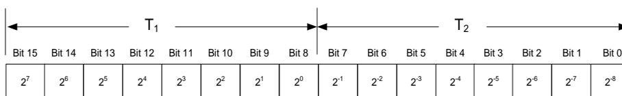
**Figure 8-9: Converting temperature data to [ $^{\circ}$ C]**
